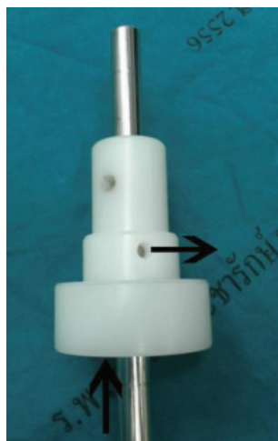
Figure 9 Airflow from the bottle through the space and side holes
